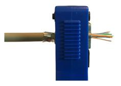
Release the tool ratchet mechanism and remove the terminated plug from the Fast-Fit Crimping Tool.
