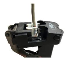
4. Fully squeeze together the handles of the KJ termination tool so that the excess wire is trimmed.
