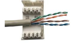
4. Punch down the wires using a Krone type or 110 style termination tool.
