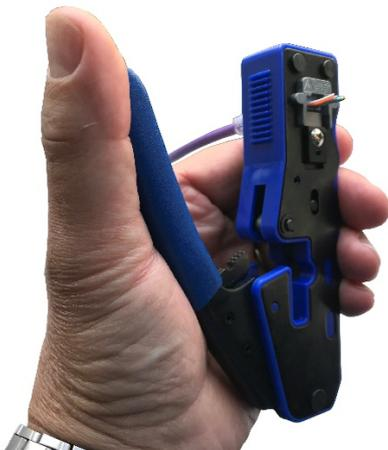
10. Release the pressure on the handles and remove the terminated plug from the Fast-Fit Crimping Tool.
