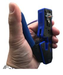
9. Release the pressure on the handles and remove the terminated plug from the Fast-Fit Crimping Tool.
